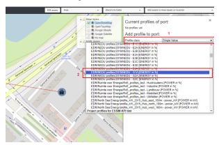
To set the value of 20 kWh heating demand per year, enter 20 in the *Multiplier* field (nr.1), and choose *Energy in kWh* from the *Quantity and Unit* dropdown menu (nr.2). To save the changes, click the *Add* button (nr.3).
